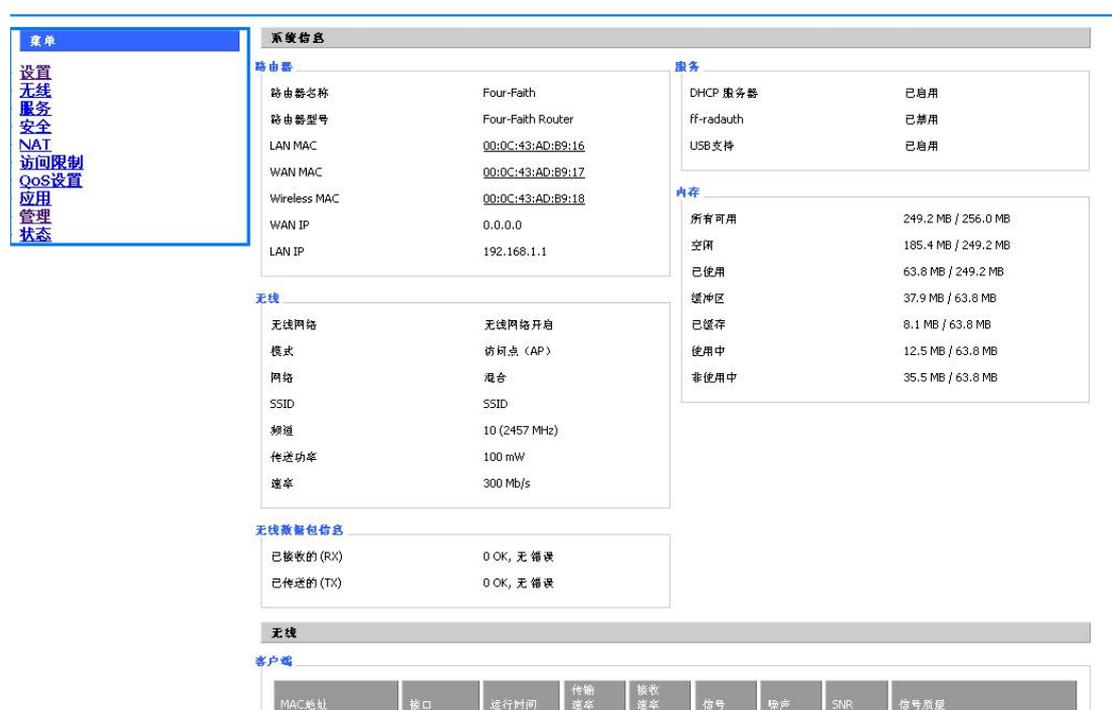
The screenshot shows the router's configuration interface. On the left is a sidebar menu with options like '设置' (Settings), '无线' (Wireless), '服务' (Services), '安全' (Security), 'NAT', '访问限制' (Access Control), 'QoS设置' (QoS Settings), '应用' (Applications), '管理' (Management), and '状态' (Status). The main content area is titled '系统信息' (System Information) and is divided into several sections:
